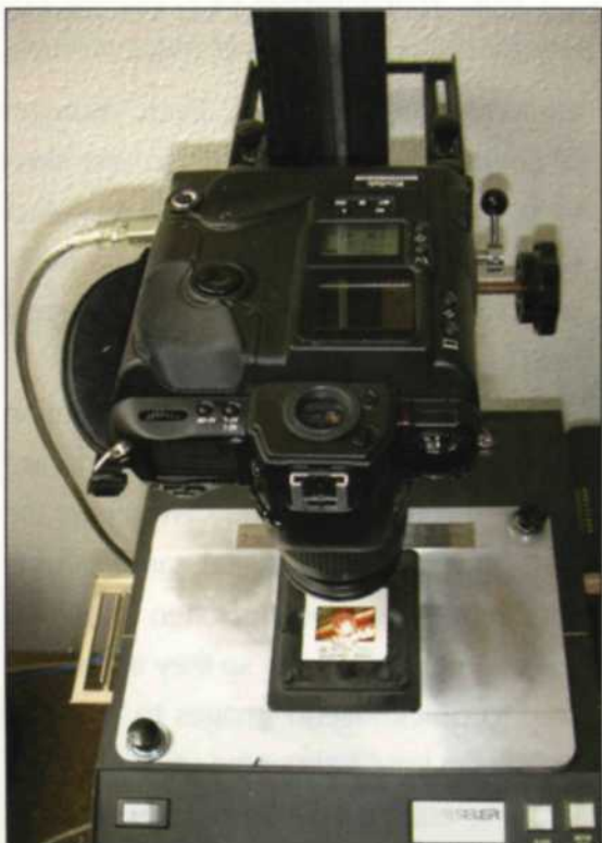
Kodak DCS660 uses a firewire cable to communicate with the computer. Images are shot and directly sent over this cable to hard disk.
