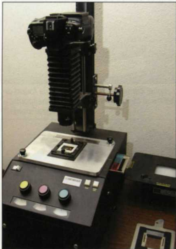
Nikon D1 digital camera mounted on a Beseler slide duplicator. Images from 35mm up to 4 x 5 can be digitized with this system.
